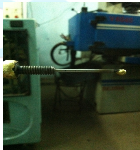
Fig. 5: Fuel Injector with 6 holes (Right side view)
